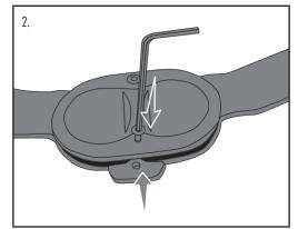
Choose the stop with the desired degrees of extension and install it on the extension stop side of the hinge. Be careful not to overtighten the screw and strip the hole.
