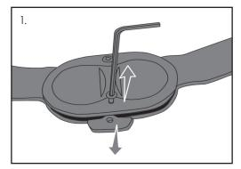
Use the included hex wrench to remove the existing hinge stops by removing the screws on both the extension stop side and flexion stop side of the hinge cover.
