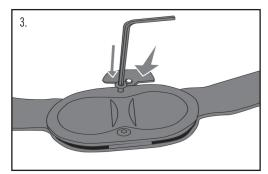
Choose the stop with the desired degrees of flexion and install it on the flexion stop side of the hinge. Be careful not to overtighten the screw and strip the hole.
